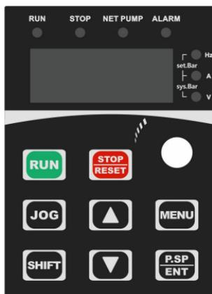
Figure1-1-1 Operation panel diagram
